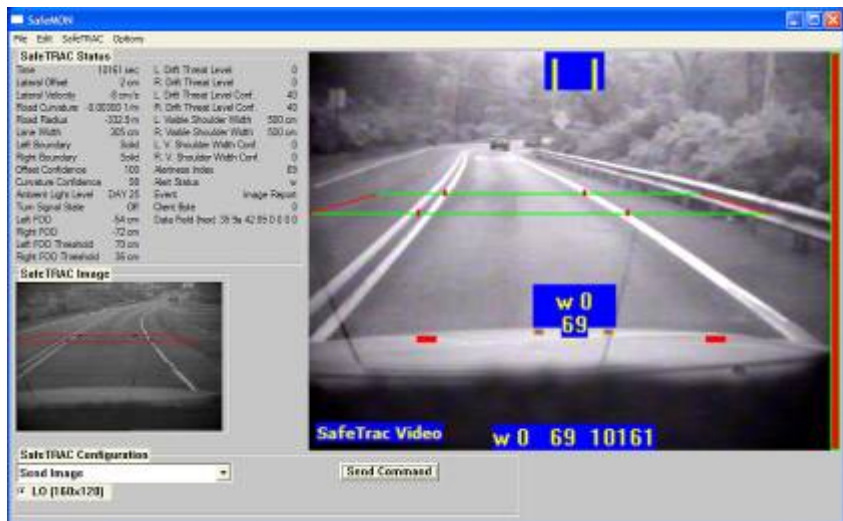
▲ SafeMON: Optional software package enables graphical view of system operation.
