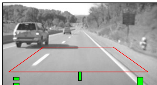
▲ Camera View: By monitoring your vehicle's position in the road ahead, SafeTRAC can determine if you are about to leave your lane.
